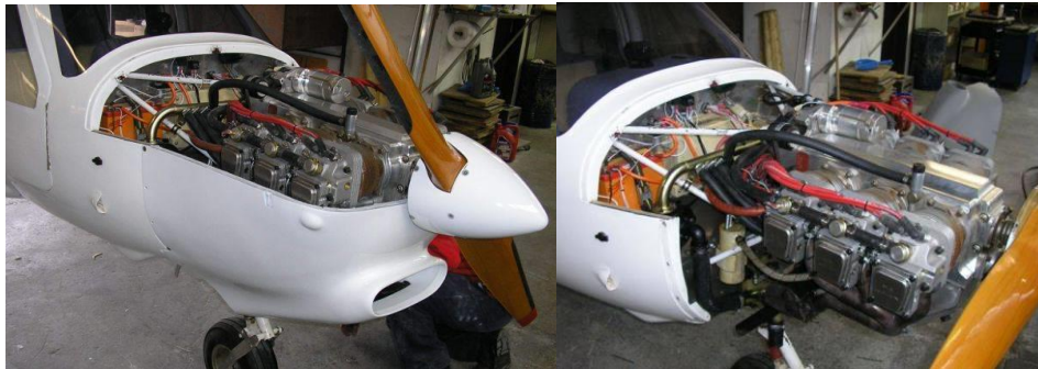
Figure 6.1: Jabiru SP 6 with the radiator mounted in front of the engine.
