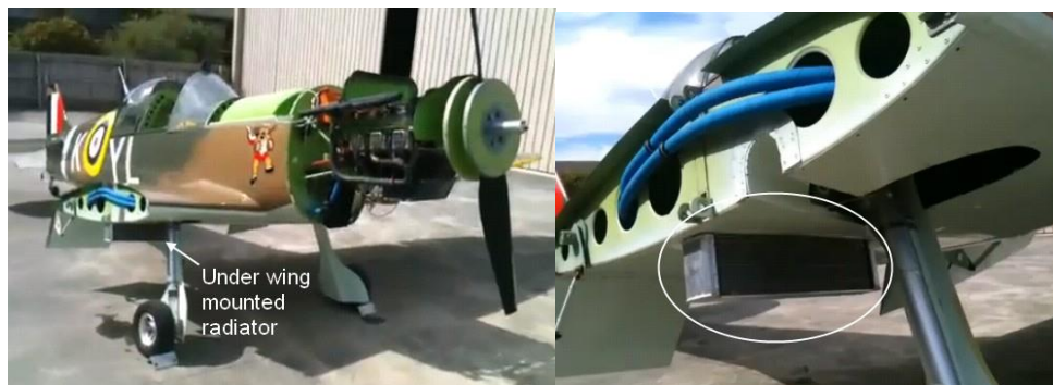
Figure 6.4: Radiator mounted under wing.
