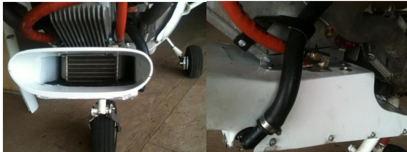
Figure 6.2: Jabiru SP 6 with the radiator plenum exposed and cowl removed
