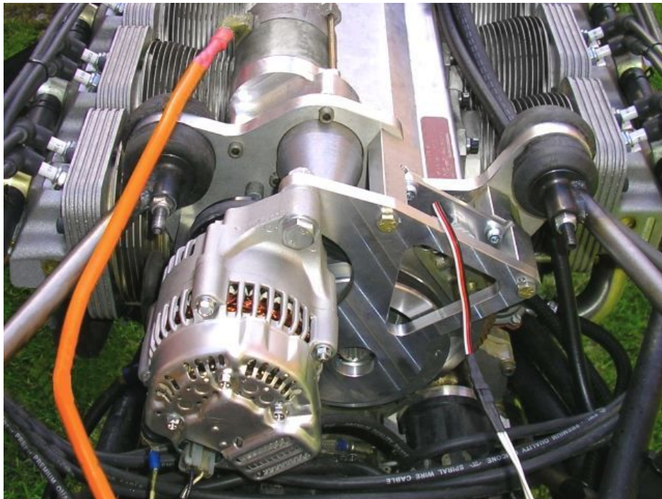
Figure 3.1.2: Completed alternator installation. E-ignition upgrade also featured (prototype engine final products differ in appearance).
